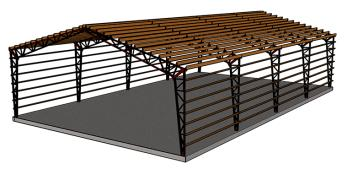
FRAMES TYPICALLY ON LARGE SPACINGS, (15' - 16') AS OPPOSED TO EVERY COUPLE OF FEET, ONE OF MANY PERKA ADVANTAGES OVER WOOD
